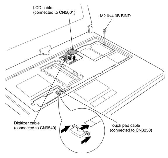
Figure 4-24 Removing the base assembly and cover assembly (1)
